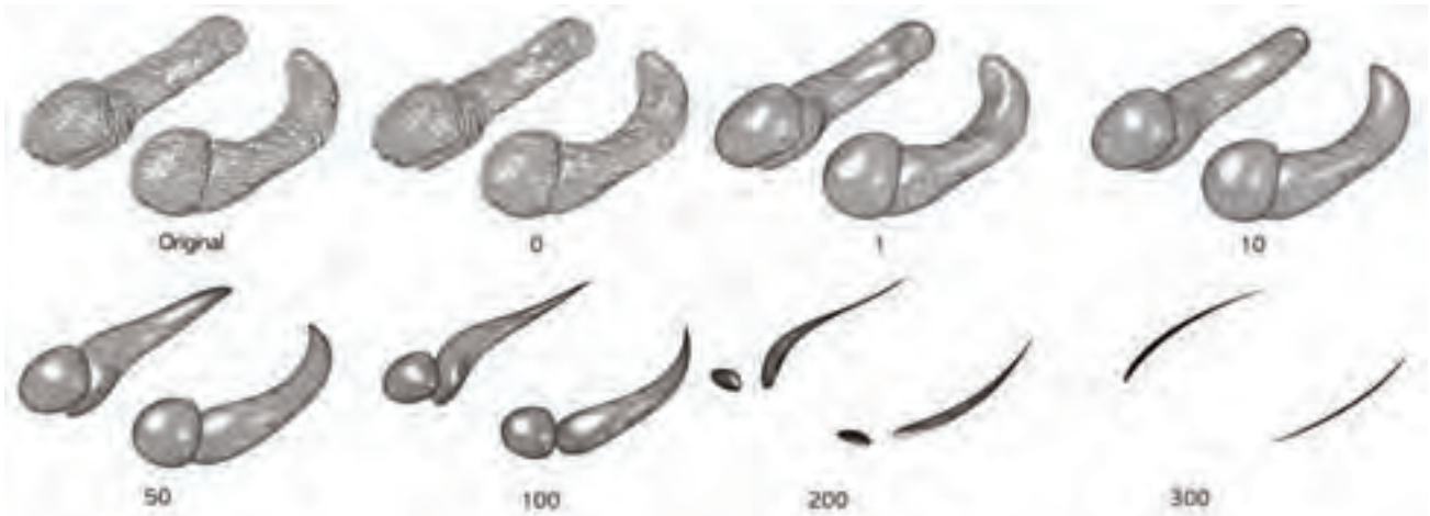
Figure 2: Sparse shape representations for different sparse parameter \lambda . As \lambda increases, the shape itself becomes sparse. For sufficiently large \lambda , it represents the skeleton of the underlying shape. \lambda = 1 is used in the study.
